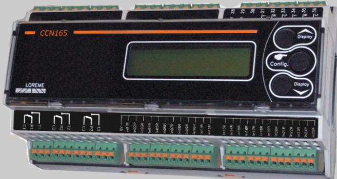
The CCN165 is a comparator of parallel digital inputs. It monitors the 2 groups of inputs to control the simultaneity of 2 mechanical organs. The output relays are activated if the code difference is too large or on an operating fault. The display allows a fast diagnostic of operating and is used for parameters setting.
